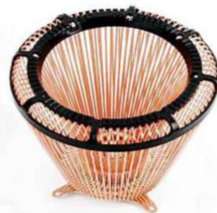
NoFan's CR-80EH can cool processors with a maximum power consumption of 80W
